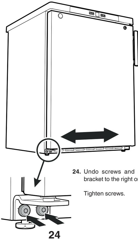
24. Undo screws and slide hinge bracket to the right or left.
