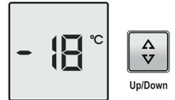
Press the **Up/Down** button, the next lower temperature value in the temperature display will light up.
