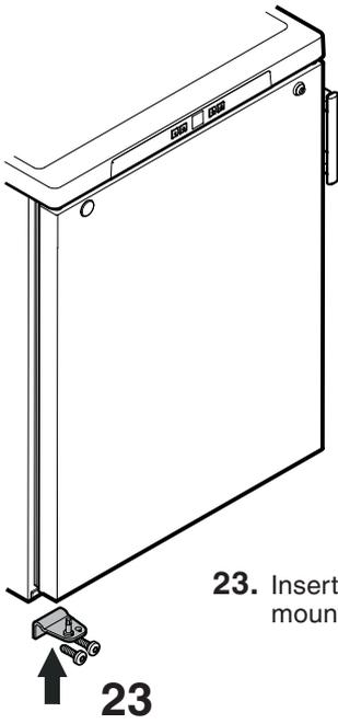
23. Insert hinge bracket in lower door mounting and screw into place.
