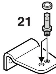
21. Transfer pin on hinge bracket to the opposite side.
