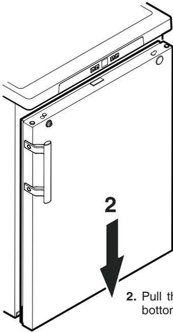
2. Pull the door out at the bottom and lift off.
