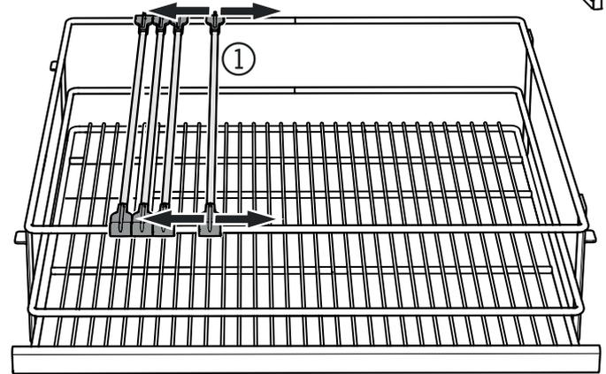
Lock the bottle holder in the required position on one of the support bars.
