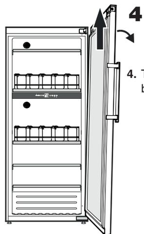
4. Tilt door slightly to the side and remove by lifting upwards.
