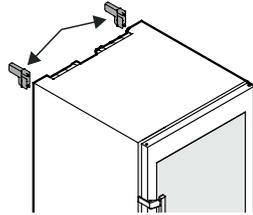
Fit the spacers to the back of the appliance on the left and right at the top.
