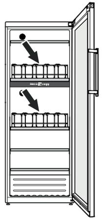
Slide the support bars ① into the required position.
