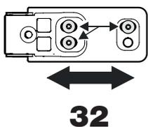
**32.** Undo screws and slide hinge bracket to the right or left.
