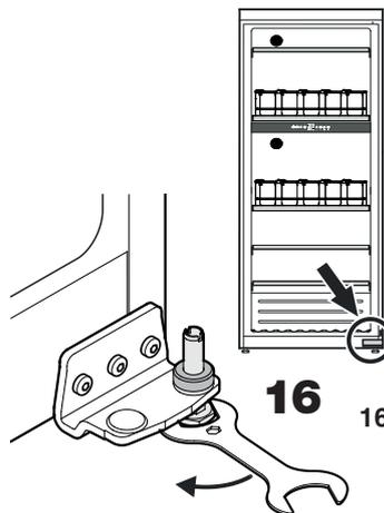
16. Undo adjustable foot with the spanner provided.
