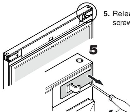
5. Release cover with a small screwdriver and remove.
