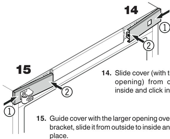
14. Slide cover (with the smaller opening) from outside to inside and click into place.
