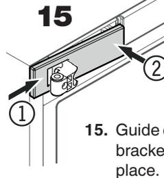
15. Guide cover with the larger opening over the hinge bracket, slide it from outside to inside and click into place.
